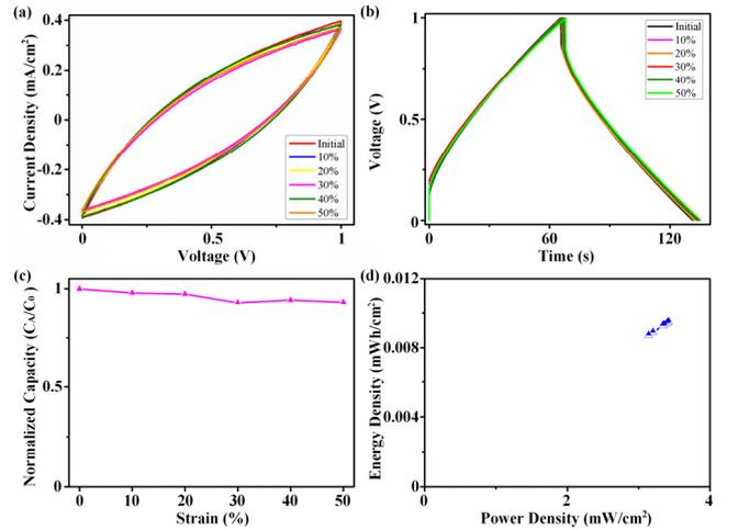
Figure 6: (a) CV curves, (b) GCD curves, (c) normalized specific capacity and (d) Ragone plot of compressible supercapacitor at different strains. Scan rate:  $100 \text{ mV/s}$ , charge/discharge current:  $1.2 \text{ mA}$ .
