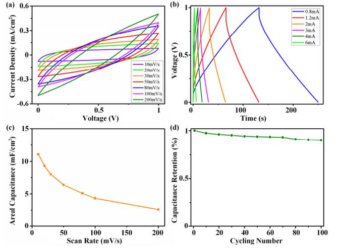
Figure 5: Electrochemical characterization of the supercapacitor. (a) CV curves, (b) GCD curves, (c) calculated areal capacitance and (d) cycling tests at  $100 \text{ mV/s}$  of the device.
