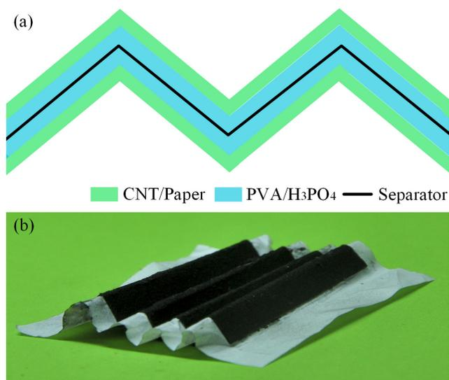
Figure 1: (a) Schematic diagram and (b) optical image of compressible solid-state supercapacitor based on folded structure.
