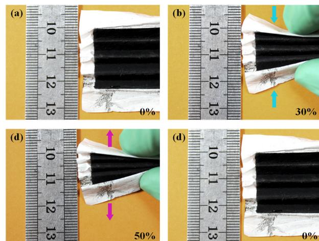
Figure 4: Real-time optical images of a supercapacitor showing the compressing and recovering process without any structural damage.
