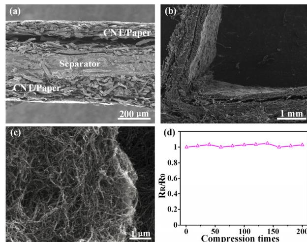
Figure 3: (a) SEM image of the cross section of the compressible supercapacitor. (b) Enlarged view of the folded structure. (c) SEM image and (d) the variation of electrical resistance of CNT/paper electrode in the first 200 compressing–releasing cycles.
