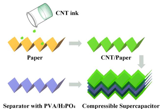
Figure 2: Fabrication flow process of compressible supercapacitor, consisting of folded CNT/paper electrode, PVA/H<sub>3</sub>PO<sub>4</sub> electrolyte and NKK TF44 separator membrane.
