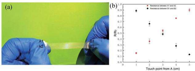
Fig.5: (a) Photograph of the 1D location sensor; (b) The relative resistance ( $R/R_0$ ) as a function of the distance from electrode A.
