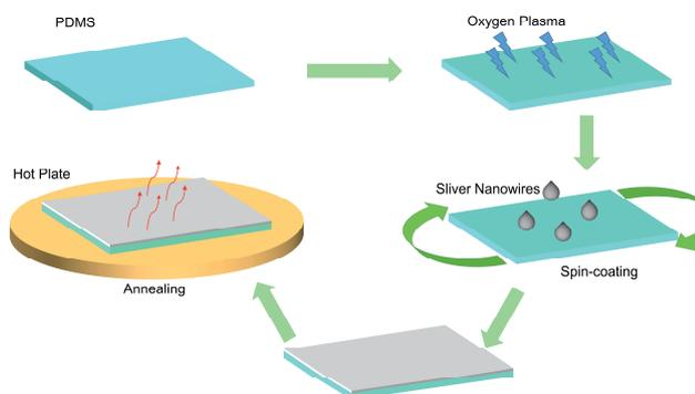
Fig.2: Schematic of the fabrication process of the PDMS/AgNWs film.
