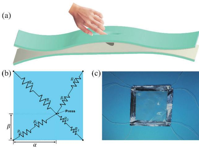
Fig.1: (a) The schematic and working mechanisms of the location sensor; The circuit schematic (b) and real photo (c) of the device.
