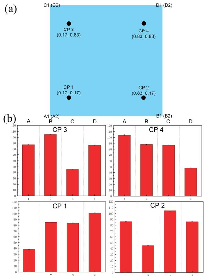
Fig.6: (a) The four contact points on the 2D location sensor; (b) The resistances of the four pairs of electrodes corresponds to four contact points were tested.
