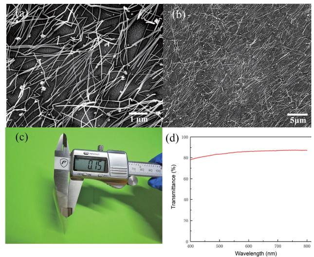
Fig.3: (a) and (b) SEM images of the AgNWs on the PDMS surface; (c) The thickness of the PDMS/AgNWs film; (d) Optical transmittance spectra of the PDMS/AgNWs film.
