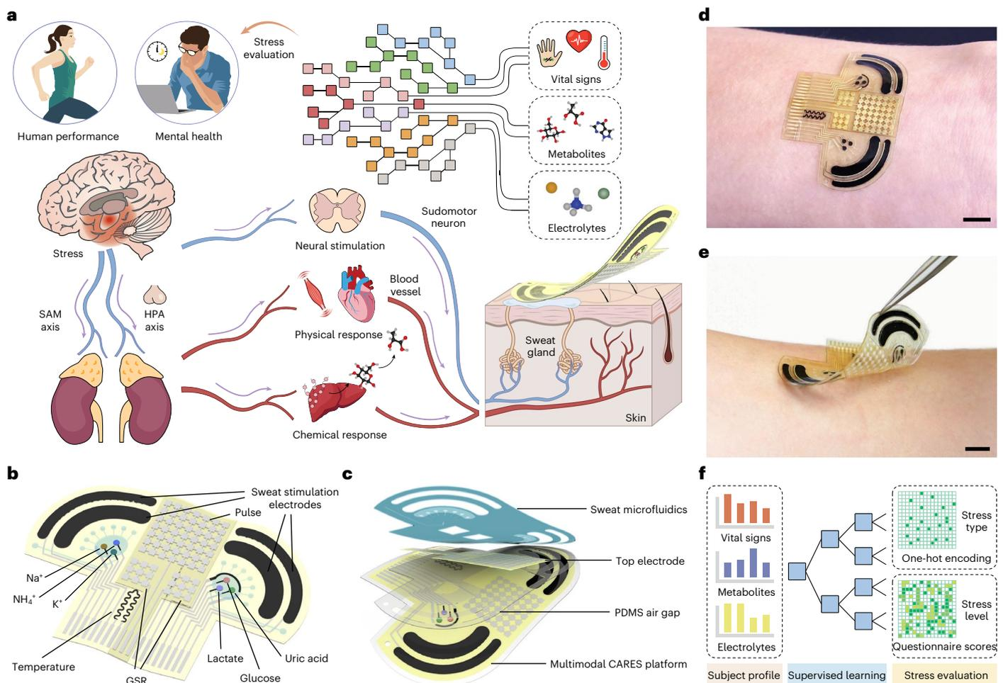
**Fig. 1 | CARES for stress response monitoring.** **a**, Illustration of the CARES that continuously monitors multimodal physiological and biochemical responses from skin and performs artificial-intelligence-powered stress assessment. **b**, Schematic of the flexible CARES sensor patch and main functionalities: vital sign monitoring, sweat stimulation and sampling and key metabolite and electrolyte
